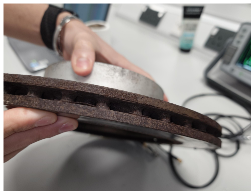
Figure 2 Brake disc (Sean D, 2024)
