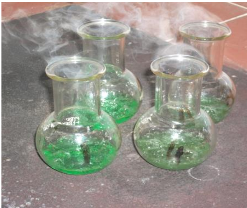
Figure 19, Photograph of samples dissolving on a hotplate
