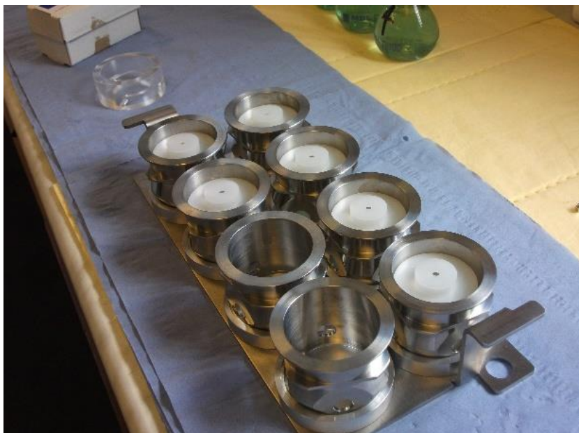
Figure 21, Photograph of receptacles before loaded into the X-ray Fluorescence Spectrometry analyser
