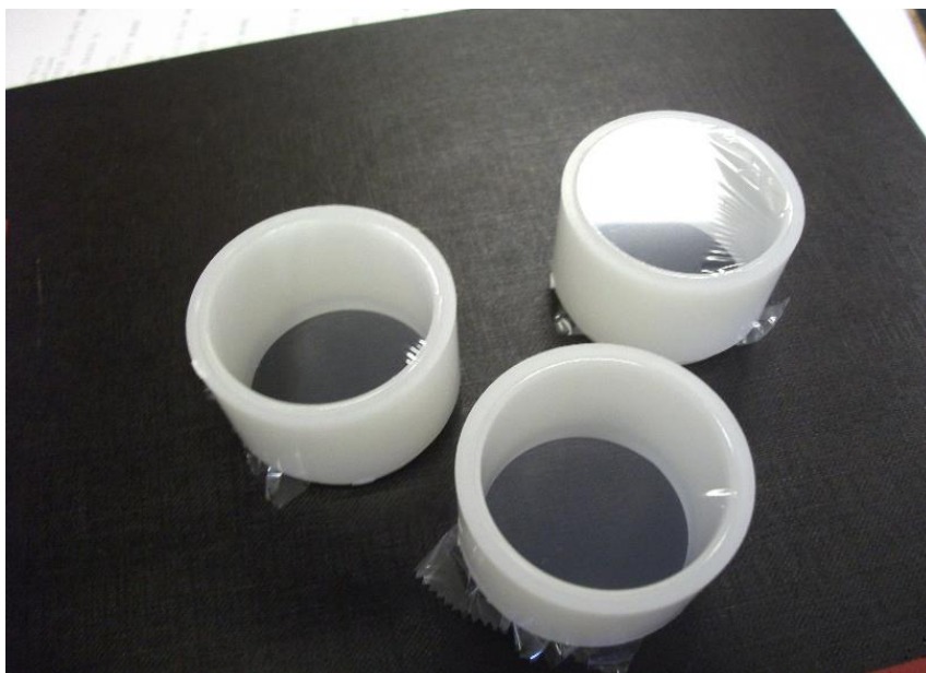
Figure 20, Photograph of sample receptacles which are loaded into the X-ray Fluorescence Spectrometry analyser
