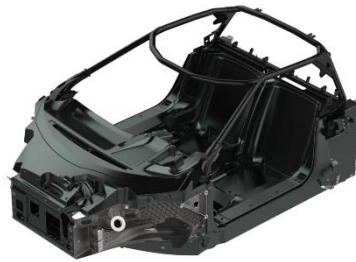
Figure 1: Carbon Fibre Passenger Cell of the 2017 Ford GT. (6 Just-Revealed Secrets About the 2017 Ford GT, the Most Anticipated Supercar of the Decade - Maxim, 2017)
