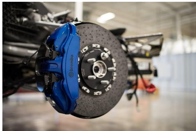
Figure 2: 2017 Ford GT's Brembo carbon ceramic brake disc. (Brembo på Twitter: "The #Brembo brake of the #Ford GT? Here's how they look like! #carbonceramic #theartofbraking https://t.co/n2Vqyo6iQN " / Twitter, no date)
