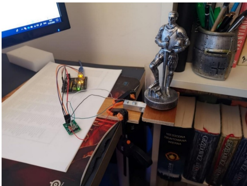
Fig.4 The example of using the scale. The statuette is placed on the load cell, and that information is registered by resistors, which send registered data to the Arduino board. Thereby, the result of the operation is printed in the console window.
