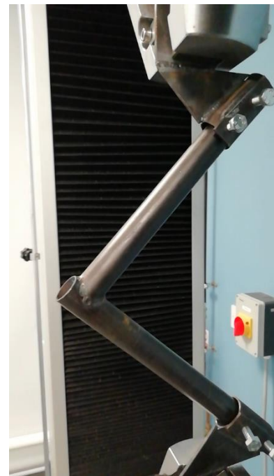
Figure 24 - Butt weld test screenshot - Oliver Gordon
