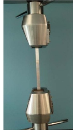
Figure 9. Workshop session 1. Installing aluminium specimen into tensile testing machine.
