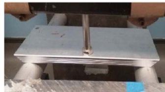
Figure 14. Workshop session 2. Destructive testing on body shell - AMC-716.
