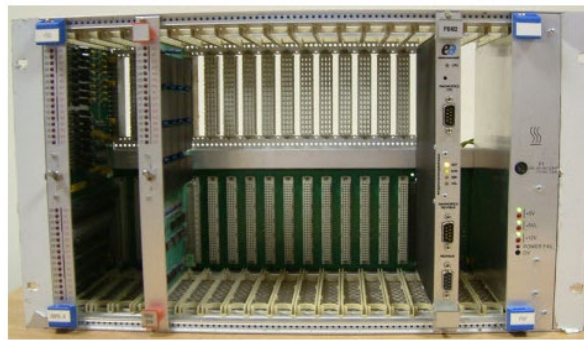
Figure 39 - Rack Mounted PLC Example
