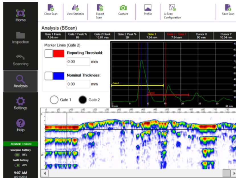
Figure 2 - example data from Scorpion2 system, showing both A-Scan and B-Scan
