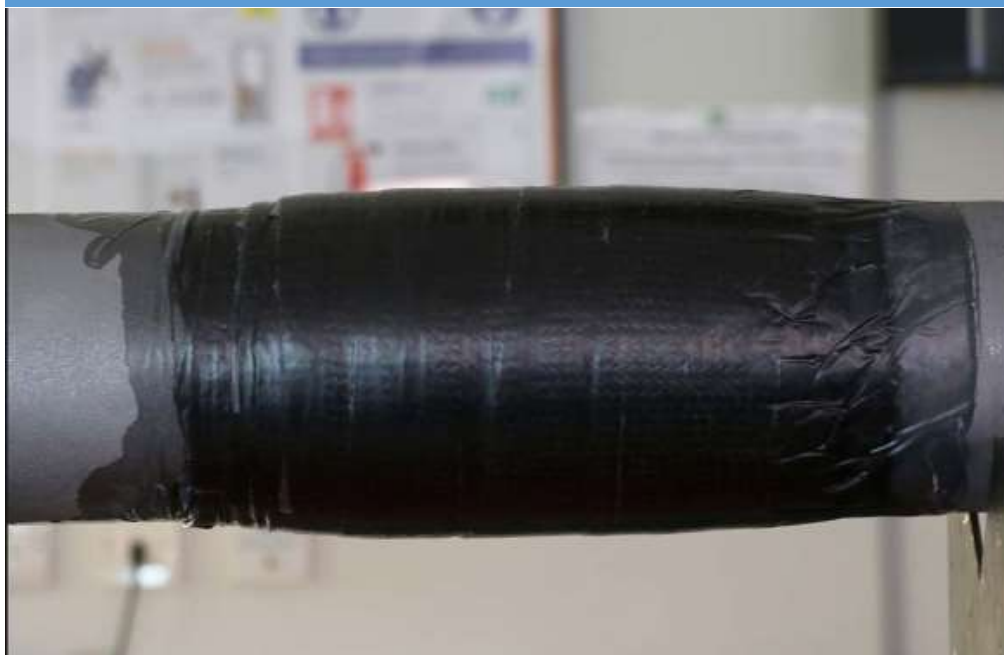
Figure 3; Composite Rap ( www.belzona.com )
