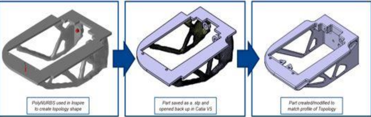
Topology results transformed back into a catia model where the analysis could be carried out. Case Study 1
