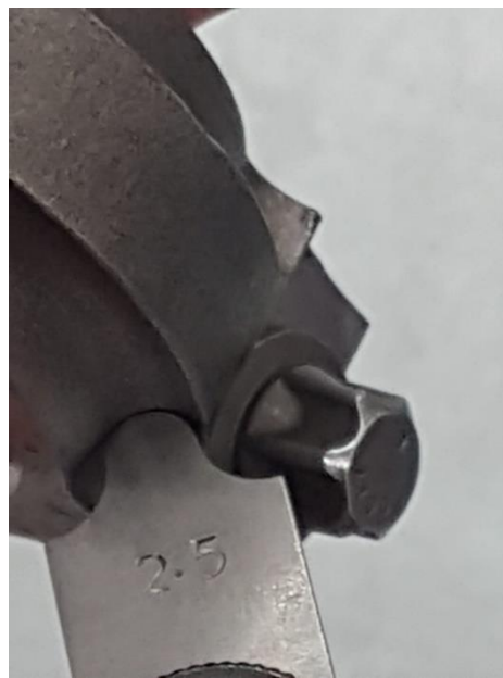
Figure 14-Measuring the radius to calculate the stress concentration
