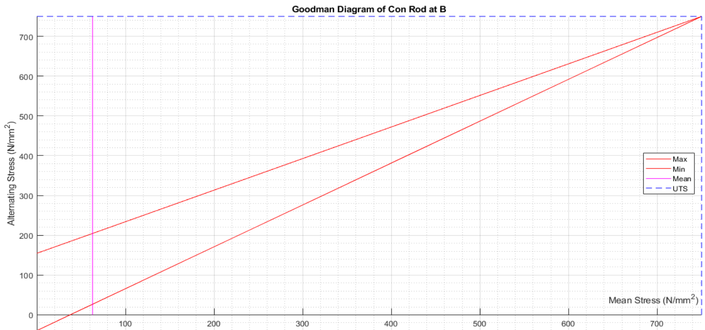
Figure 10-Goodman Diagram of con rod at point B
