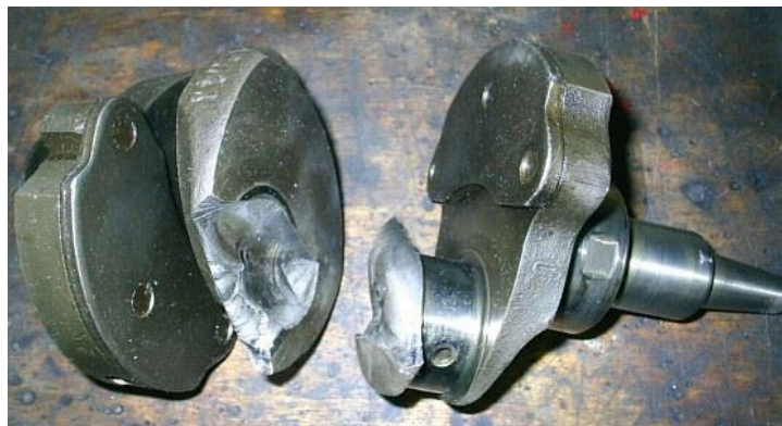
Figure 18-Image of broken crankshaft
