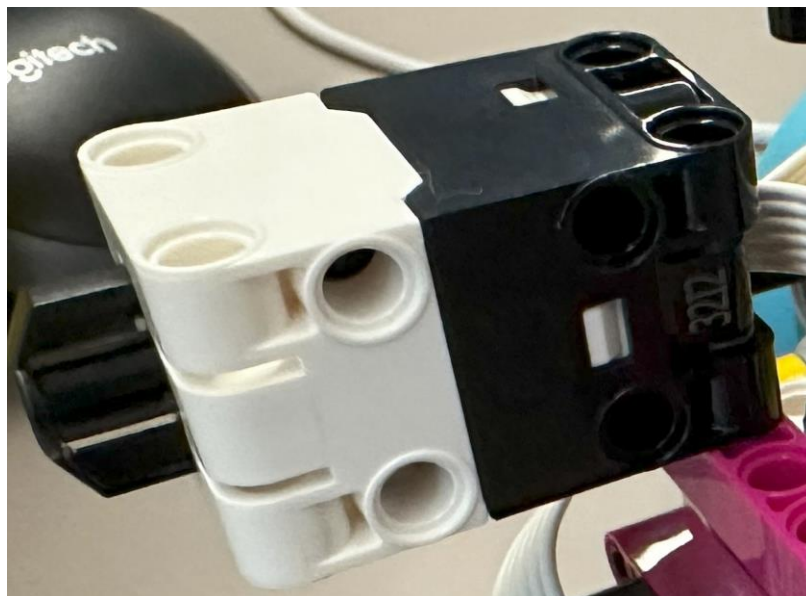
The Force Sensor – A sensor that sense force or pressure being applied
