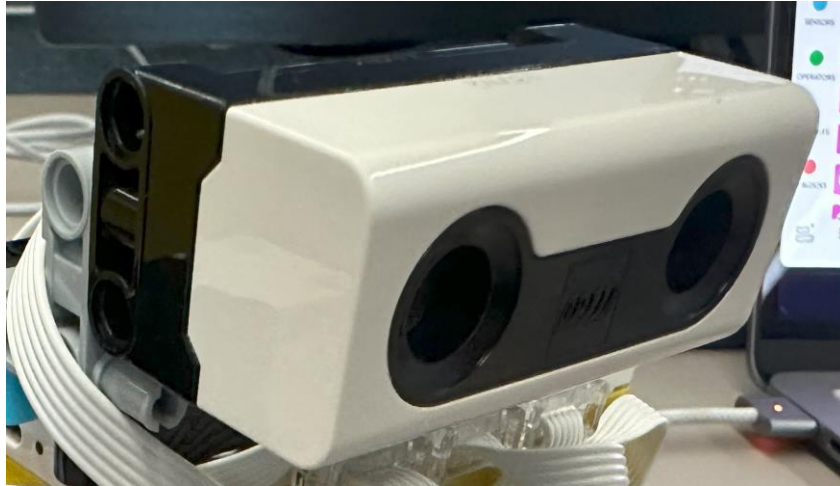
The Distance Sensor – A sensor that can gauge the distance nearby objects within its sight
