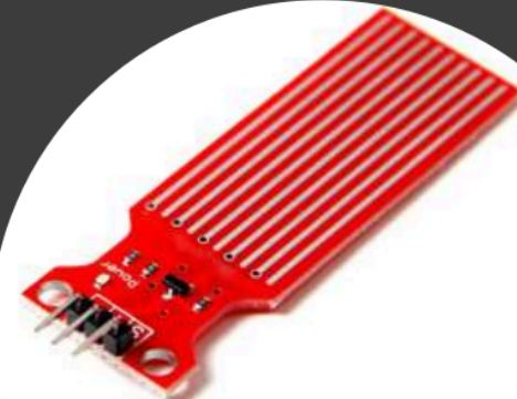
Level PCB to detect liquid level only
