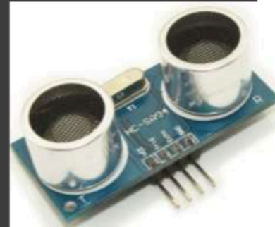
Ultrasonic sensor to detect liquid or solid substances
