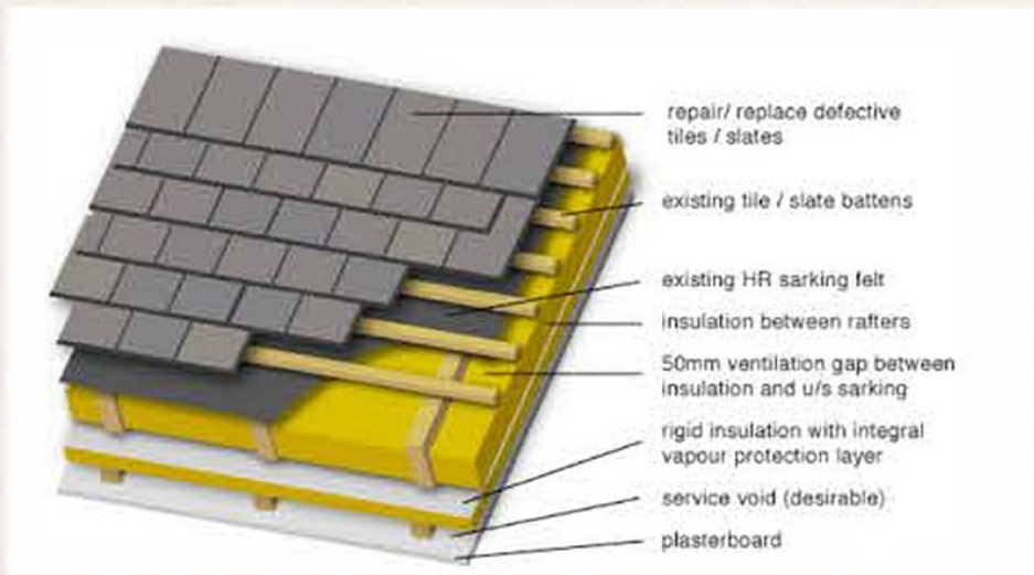
(HOUSING RETROFIT: VENTILATED PITCHED ROOF INSULATION2025)
