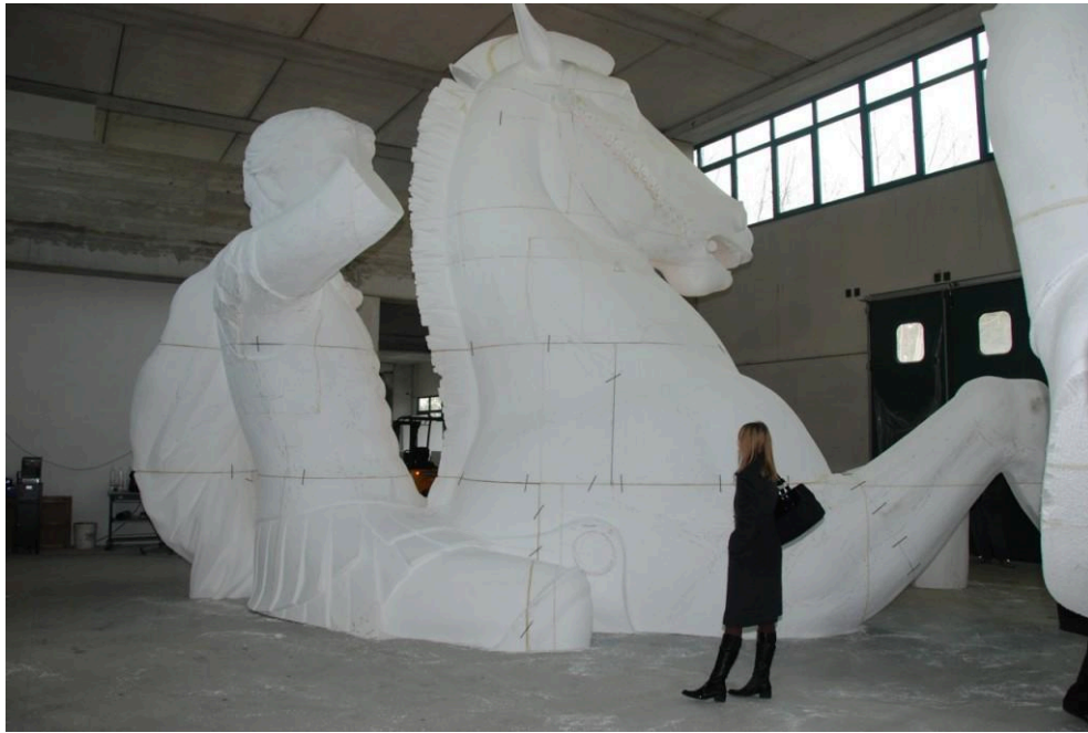
Fig. 4 The enlargement stage (Marinelli Foundry, 2008)
