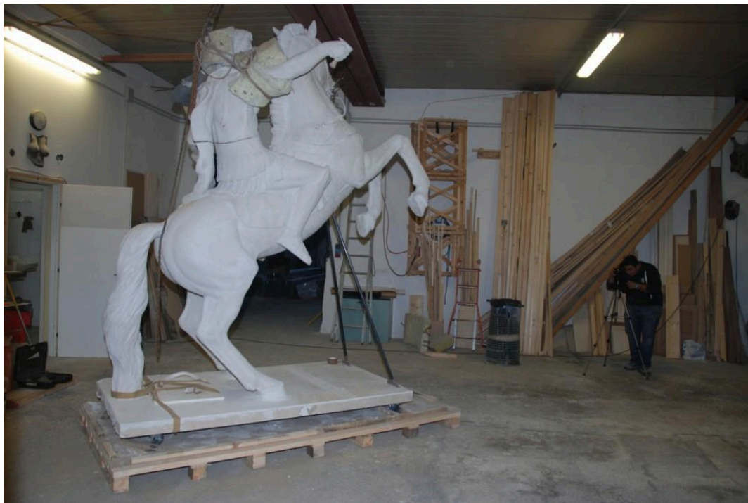
Fig. 3 The original 3.5 plaster model to be enlarged and executed in bronze (Marinelli Foundry, 2008)
