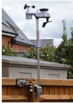
Figure 2: ACCUR8 DWS5100 5-in-1 Solar-Powered WiFi Weather Station [4]
