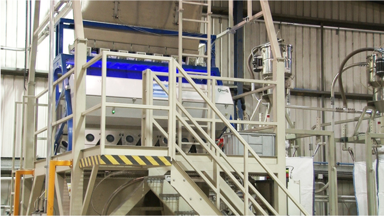
Optical colour sorting machines, utilising ultraviolet light to sort plastics by colour.
