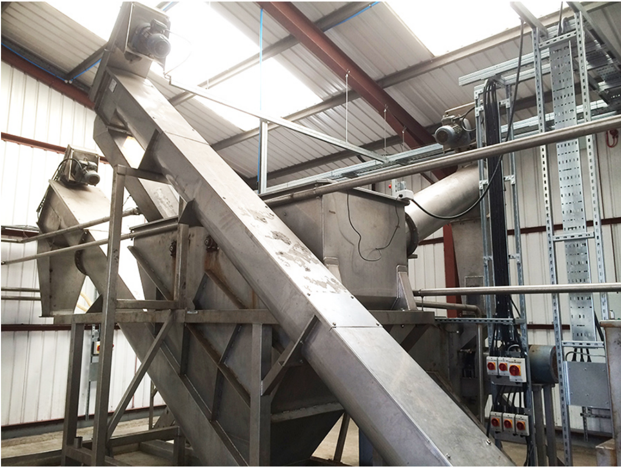
Sink-float technology, used as part of the wet separation process.
