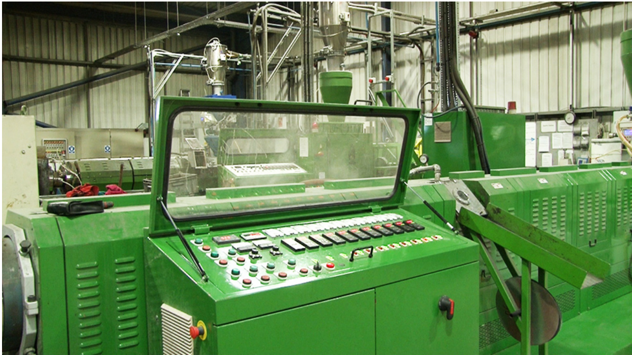
An extrusion machine, responsible for the final phase of the recycling process. Image credit: Plasgrind. (2015). Plasgran plastic recycling compounding equipment [Image]. https://plasgranltd.co.uk/wp-content/uploads/2015/10/Plasgran-plastic-recycling-compounding-equipment.jpg
