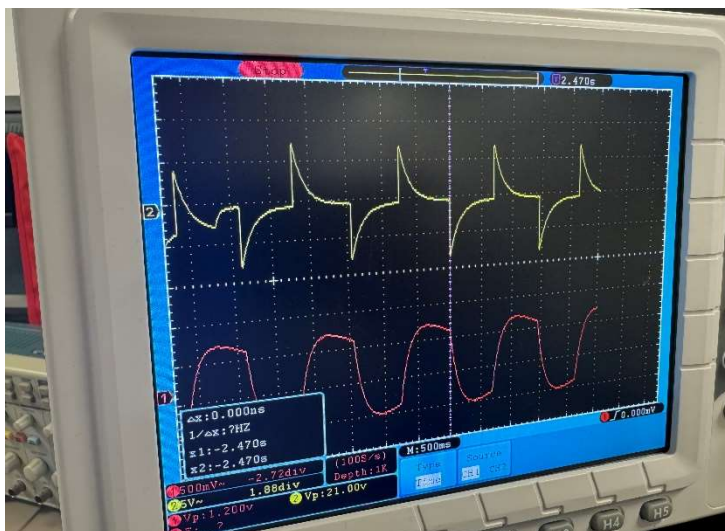
Figure 14 Graph of Capacitor (C1) voltage and output voltage against time for breadboard circuit
