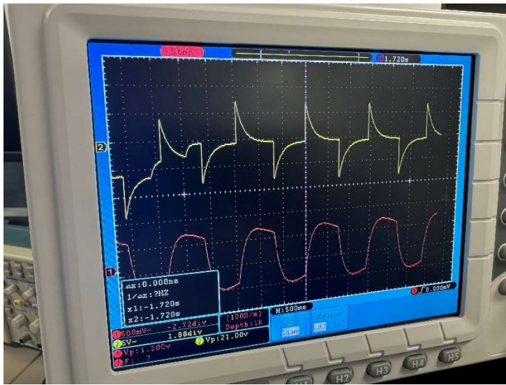
Figure 13 Graph of Capacitor (C1) voltage and output voltage against time for breadboard circuit
