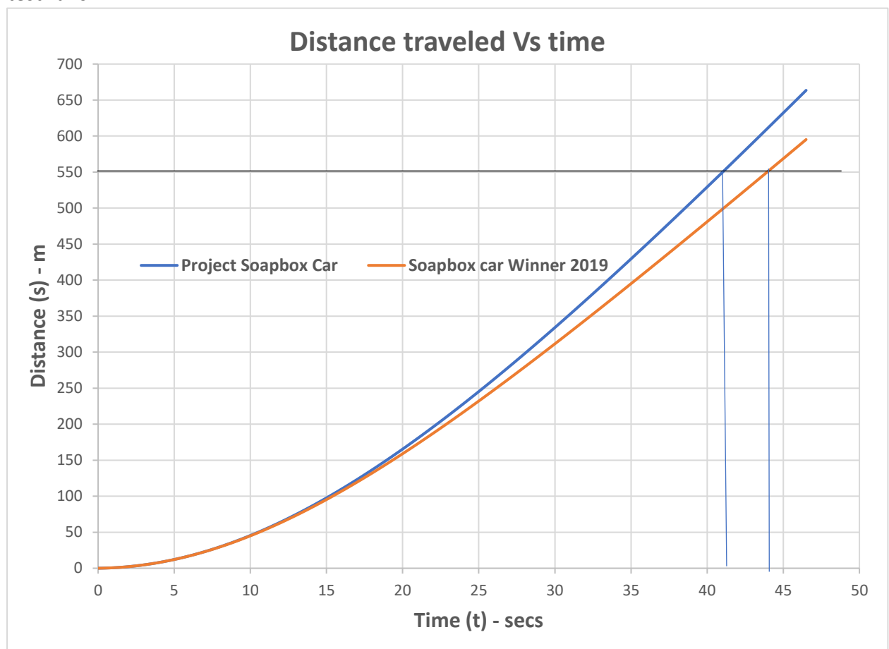
Figure 6 – Distance Vs. time - Comparison between Project soapbox car and 2019 winner Soapbox Car
