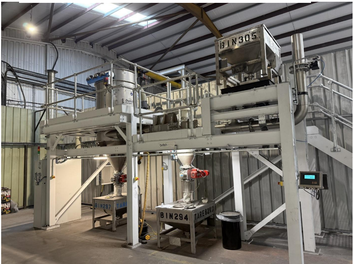
Figure 10 – British Rema Air Classification System
