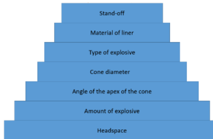
Figure 7 - Hierarchy of physical variables that affect the jet formation of a shaped charge [31].
