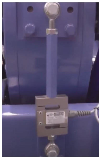
Figure 6 (strain gauge for measuring the movement of the dyno housing)
