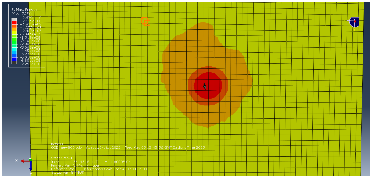
Figure 15- 800\text{m/s}^{-1} , step 18000, time 1.8\text{E}-04 , max principle, rear of plate
