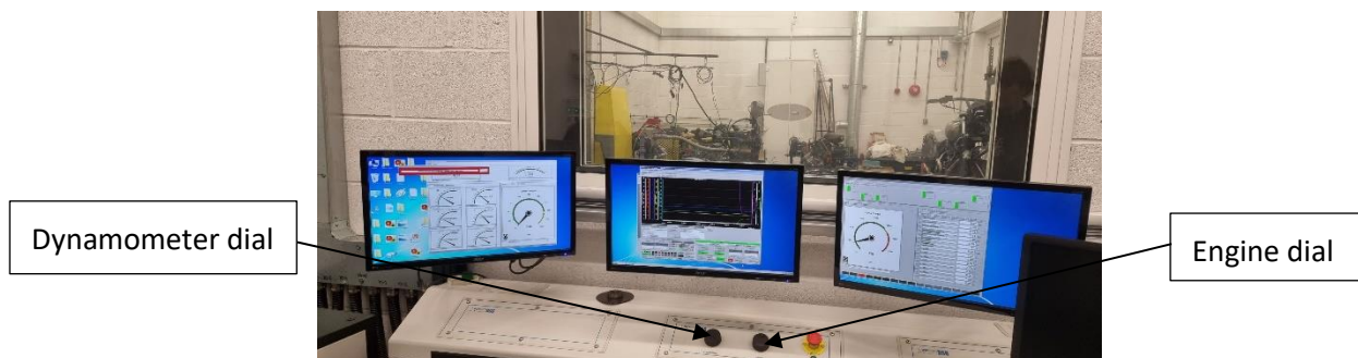
Figure 3 - Labelled photo of the control panel for the dyno.
