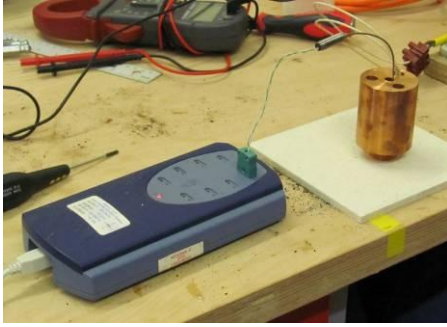
Figure 3.18 Copper Heater, TC A1 and Nico controller.
