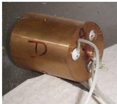
Figure 3.5 All 3 heater elements fitted to copper heater
