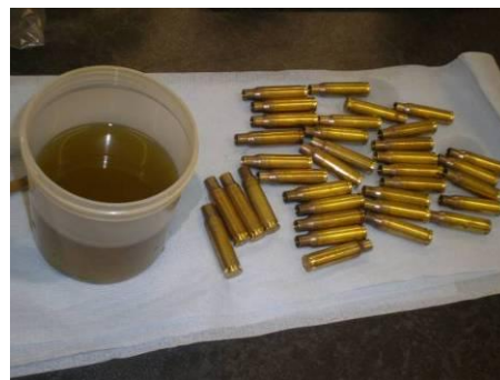
Figure 3.10 Cartridge cases (post acetone clean)
