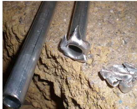
Figure 3.6 20mm of Al tube destroyed with remaining fragments shown.
