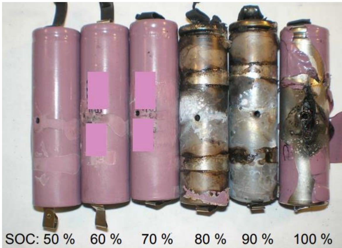
Figure 1 TIAX Nail Penetration Test (IATA, 2019).
