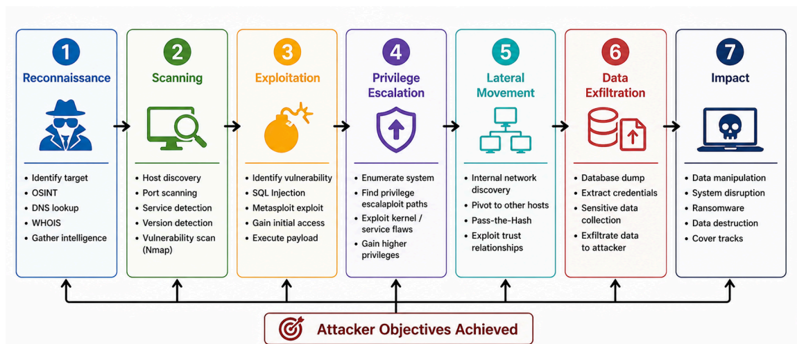
Figure 13: Illustrates the attack progression based on the Cyber Kill Chain model, demonstrating how an attacker moves systematically from reconnaissance to full system compromise and data exfiltration.
