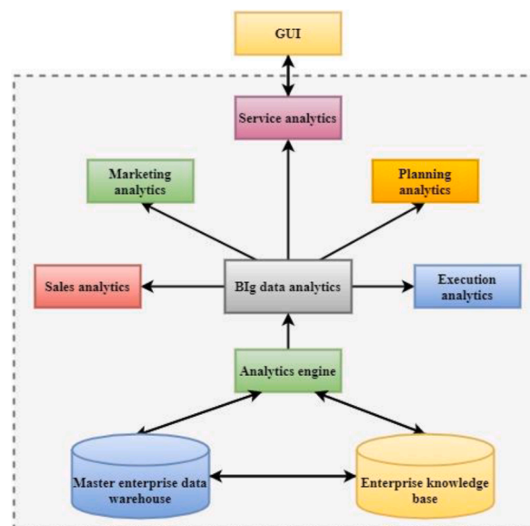
Fig. 5. Data analytics architecture of the proposed Optimized Data Management using Big Data Analytics (ODM-BDA) framework.
