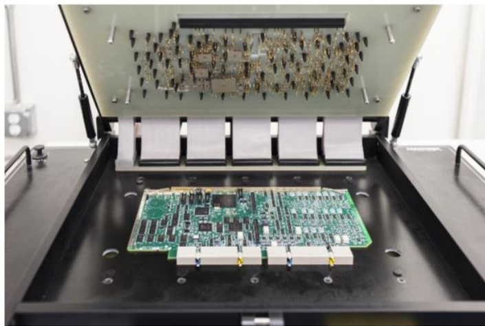
Figure 2.16 - In circuit tester (PARPRO Technologies , 2016)
