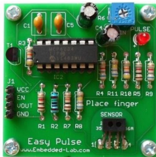
Figure 2.1 - Single sided PCB (Anon., 2013)
