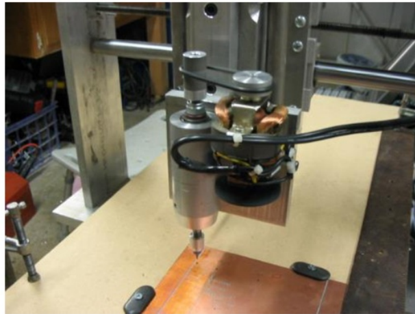
Figure 2.5 - PCB drilling machine (Kush , 2014)
