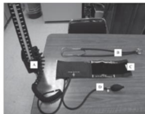
PHOTO 3.1 A mercury sphygmomanometer. (A) Mercury column with pressure gradients listed from 0 to 300 mmHg, (B) stethoscope, (C) cuff, (D) air bulb and pressure release valve for inflating the cuff.
