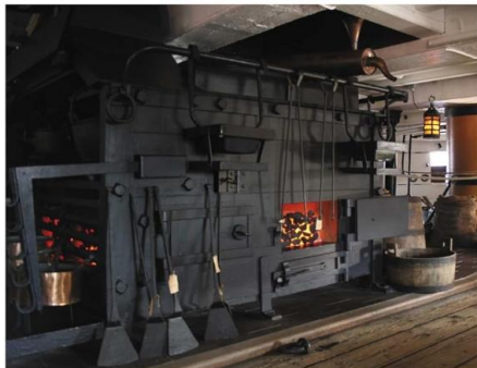
ABOVE The British pattern gun galley stove - elevated view showing fire box under baffles, heating water door and fire hearth, and rails for hoisting the fire.
