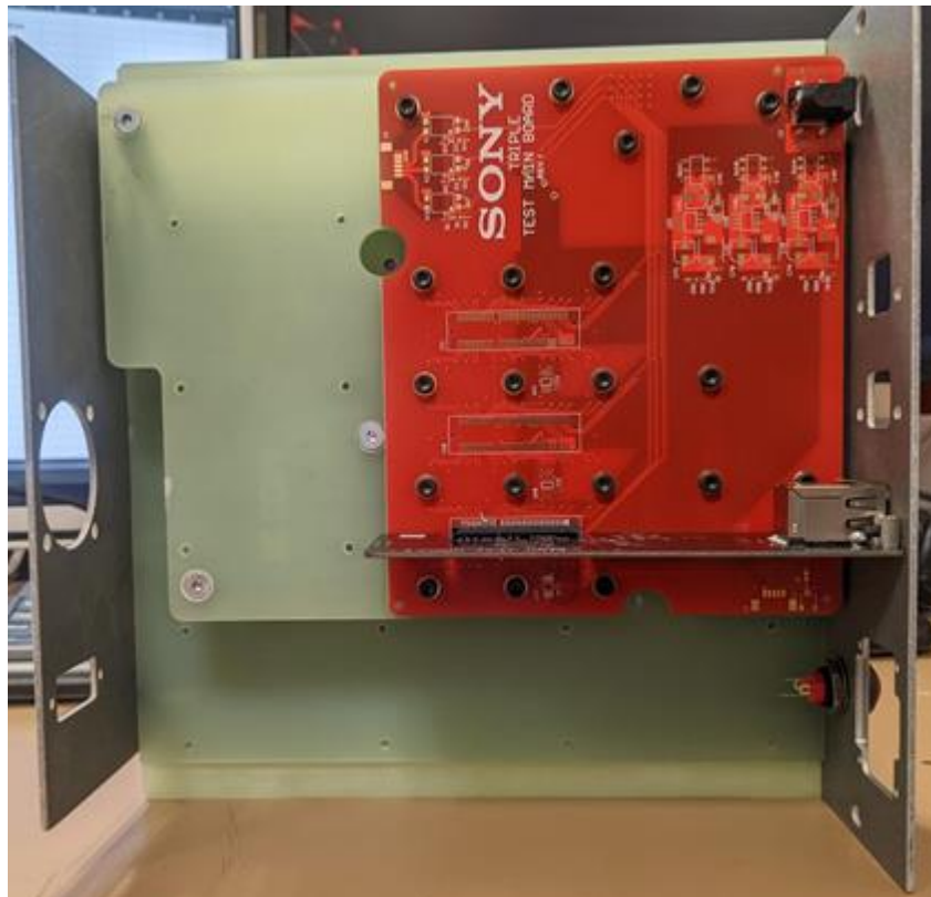
Figure 34 - Main board fitted into pinbase bottom
