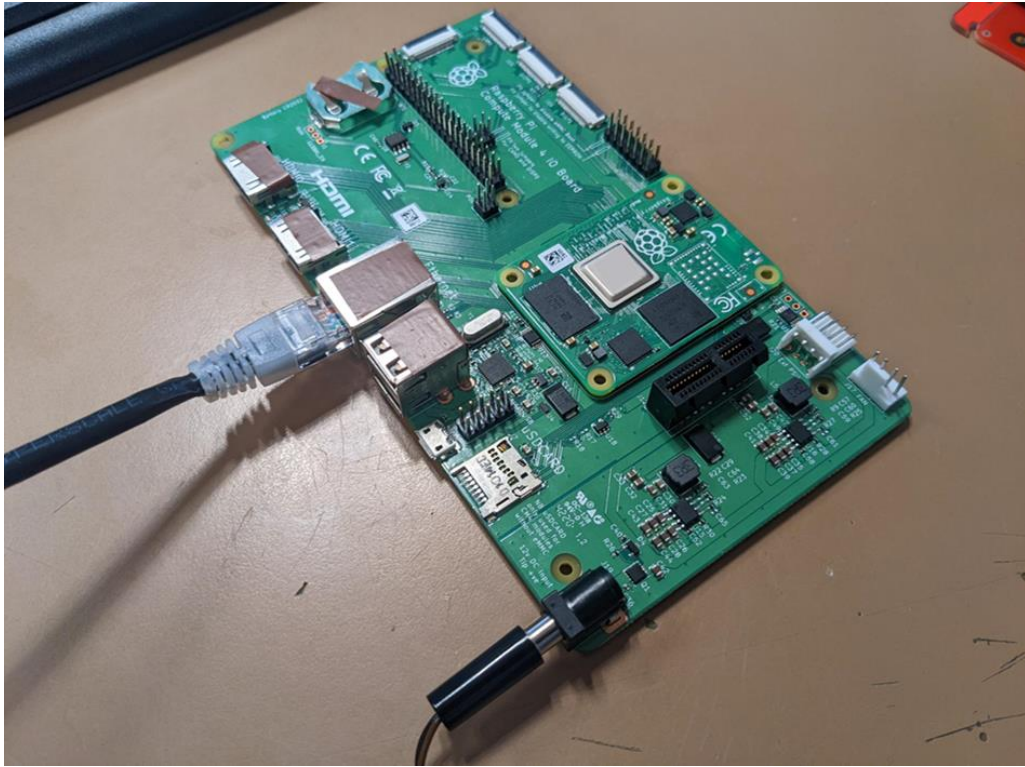
Figure 28 - Image of CM4 on CM4 IO board with ethernet connected
