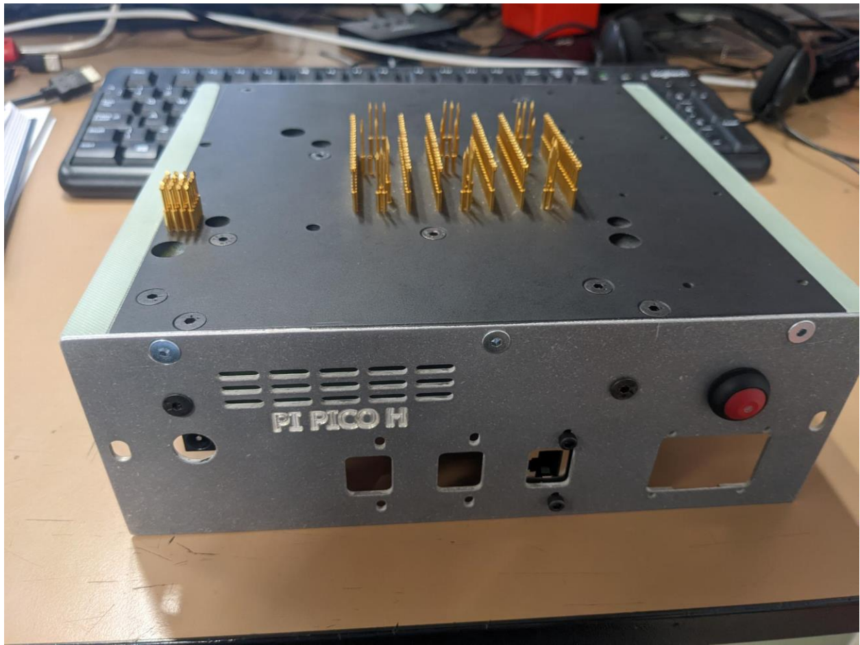
Figure 35 - Alignment of mounting holes and ethernet on front panel of pinbase
