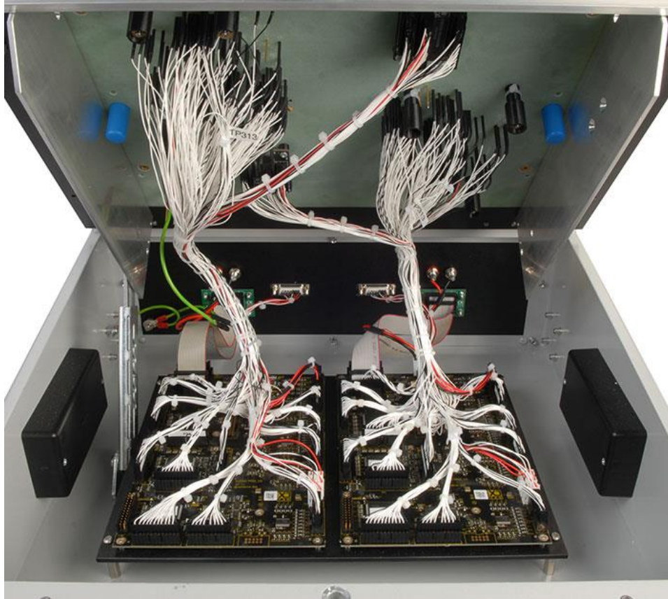
Figure 5 - Image of test jig with soldered wire connections to pin receptacles [5]
