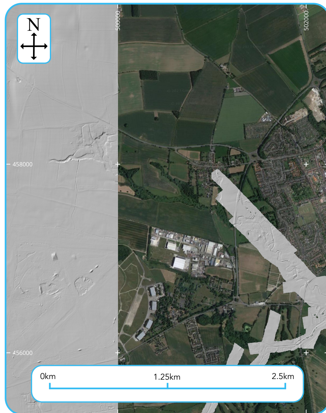
2014 - Intermittent coverage of 1m and 0.25m LiDAR composite DTM data becomes available from surveys completed by the Environment Agency [DEFRA] in 2005, 2006 and 2014.
