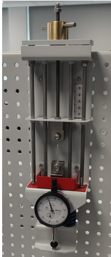
Figure 1 - Image of the Tensile Tester used
