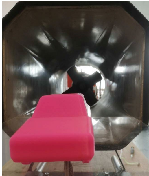
Figure 22 - 3D Printed MIRA Reference Geometry in Small Scale Wind Tunnel.
