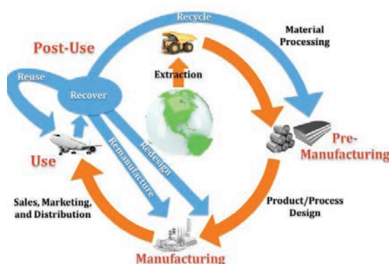
Fig. 5. Closed-loop material flow diagram of 6R elements and the four life-cycle stages.
