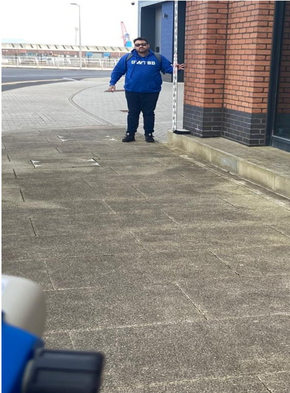
Figure 1 Levelling staff set up at Benchmark position
