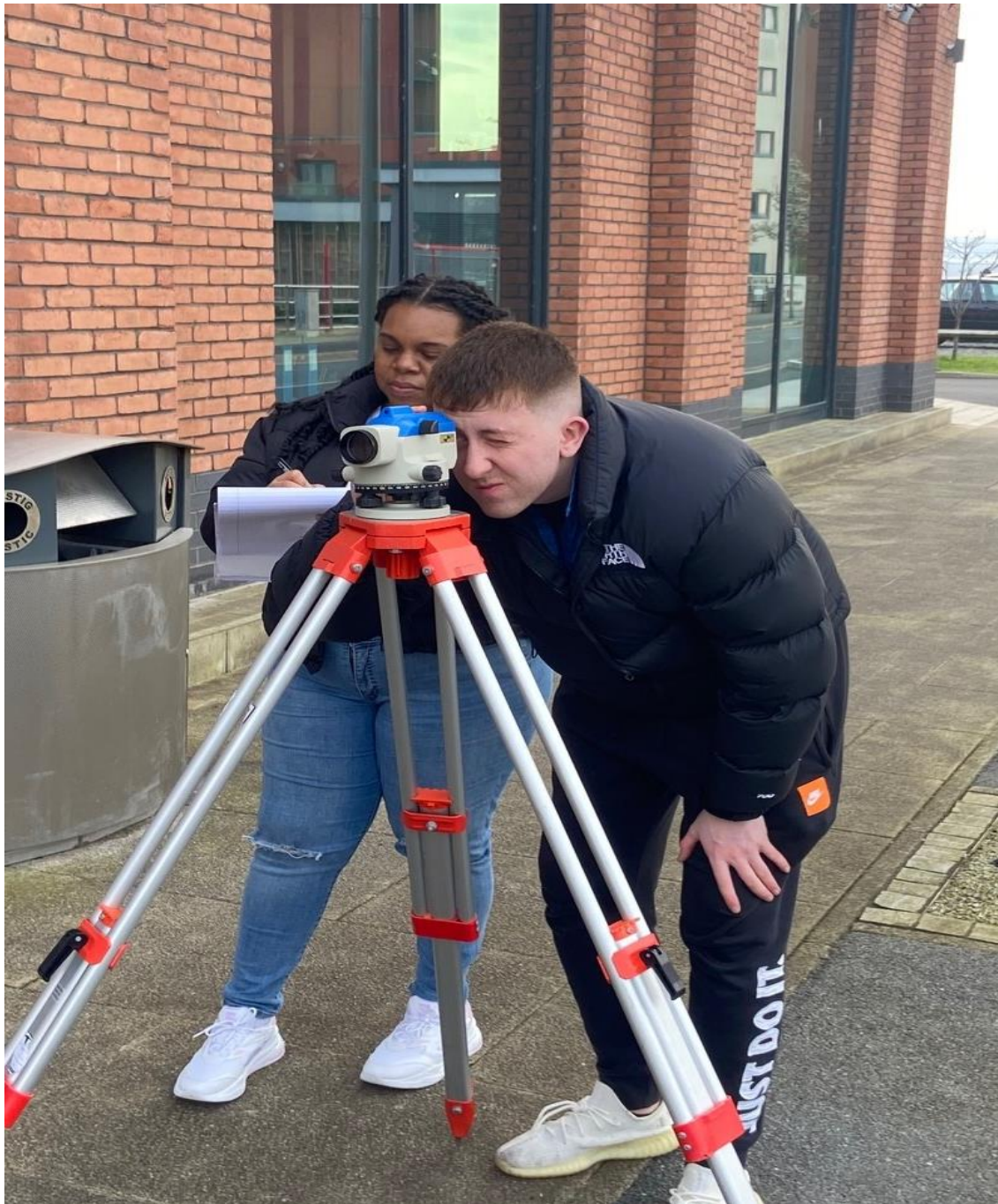
Figure 2 Levelling instrument set up to record B.M reading
