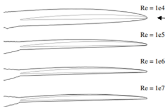
Figure 4: "Contour line of total pressure loss ( C_{pl} = 0.01 ) representing the boundary-layer shape for J=0.7 for E779A propeller at 0.7R " (Rijpkema, Baltazar and Falcão de Campos, 2016 p.8)
