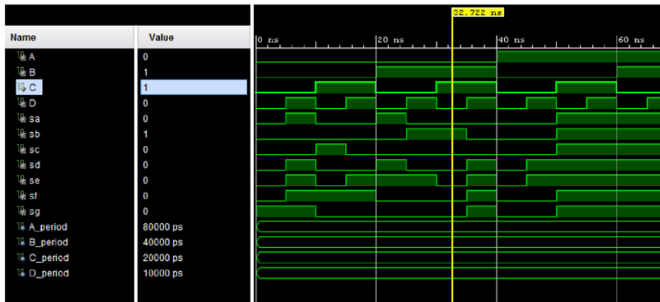
Figure 44 - BCD to 7-Segment Simulation - 6
