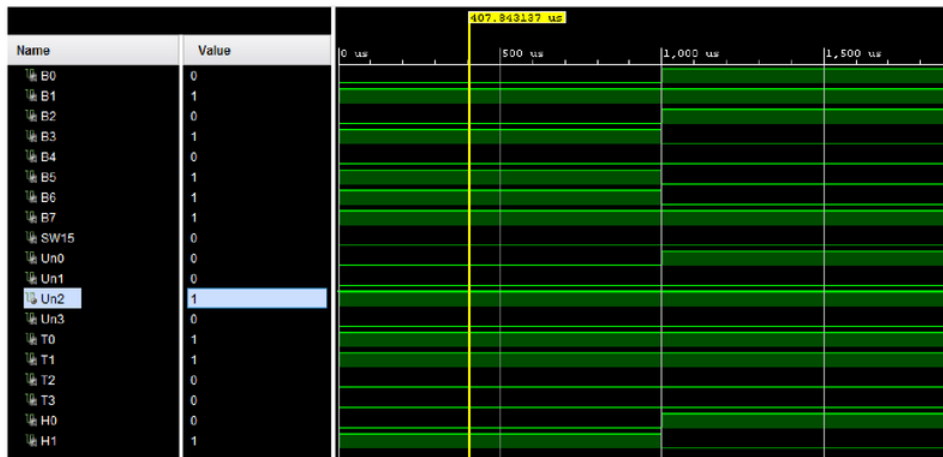
Figure 14 - Simulation of 8-bit Binary-to-BCD - 234
