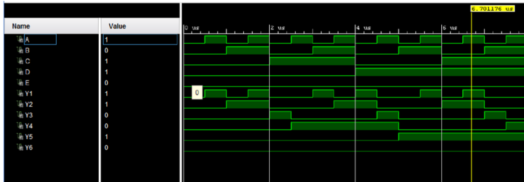
Figure 11 - Simulation of 6-bit Binary-to-BCD - 26/27 Good Analysis
