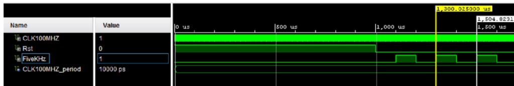
Figure 42 - 5KHz Clock Simulation
