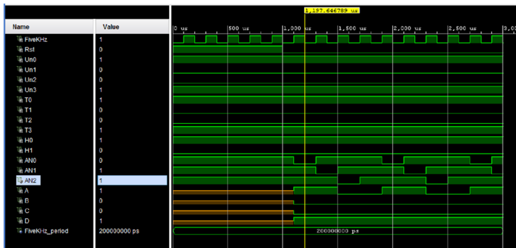
Figure 39 - 3*4-bit Mux_Demux Output - Units
