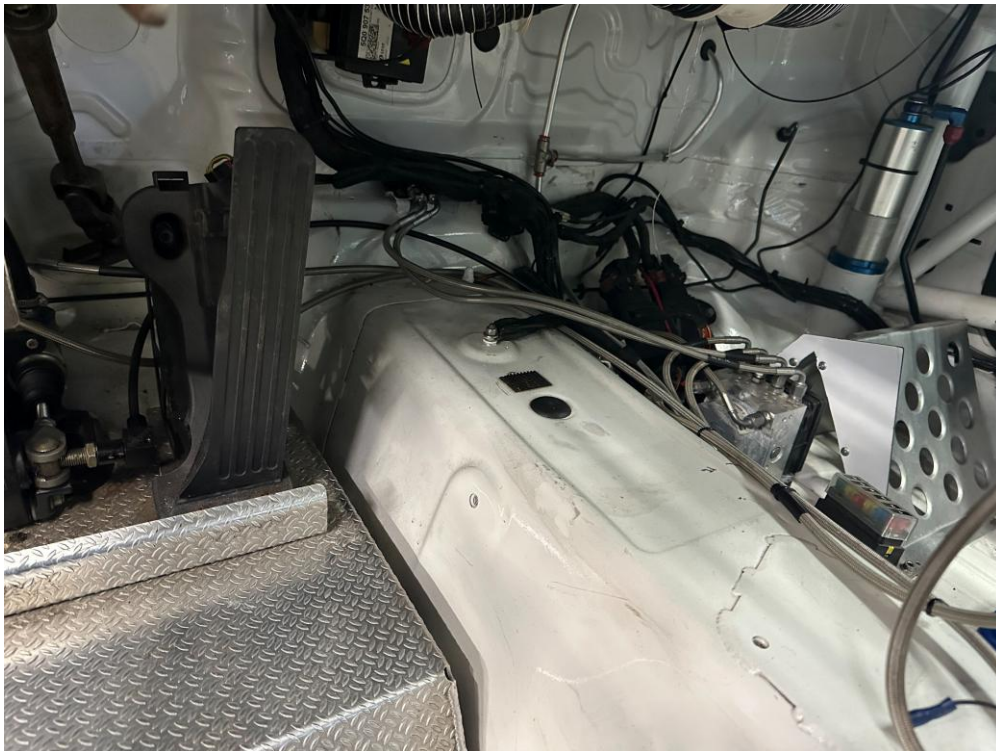
Figure 7. Transmission tunnel, internal line routing, and stripped shell structure inside the racecar cockpit, highlighting the decrease in trim, changes in packaging, and the elimination of NVH isolation for a road car.
