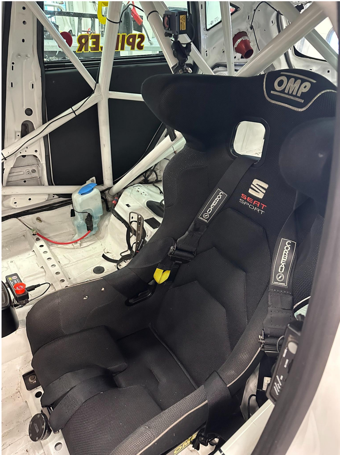
Figure 10. Driver's seat, harness and survival-cell layout, showing the race-car restraint strategy that replaces the road-car airbag and pretensioner-based safety approach.
