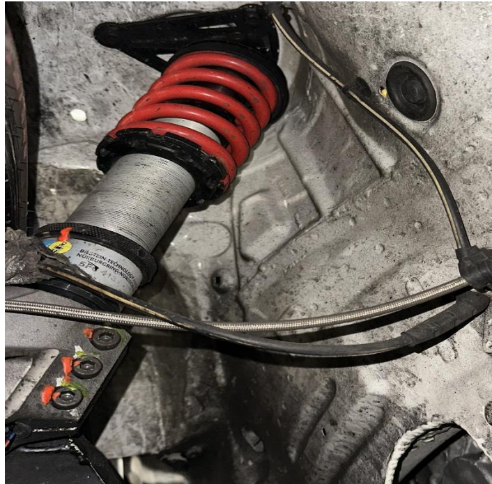
Figure 4. Front suspension wheelhouse and race damper installation, showing motorsport hardware acting through the production-derived inner wing and front hard-point region.
