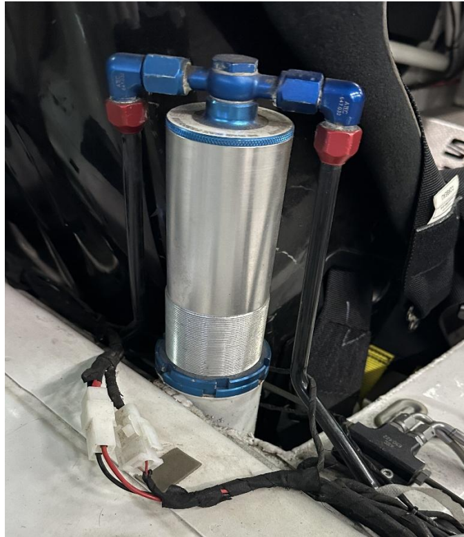
Figure 8. Rear air-jack cylinder and local body reinforcement, showing how motorsport service features require welded reinforcement within the original shell.
