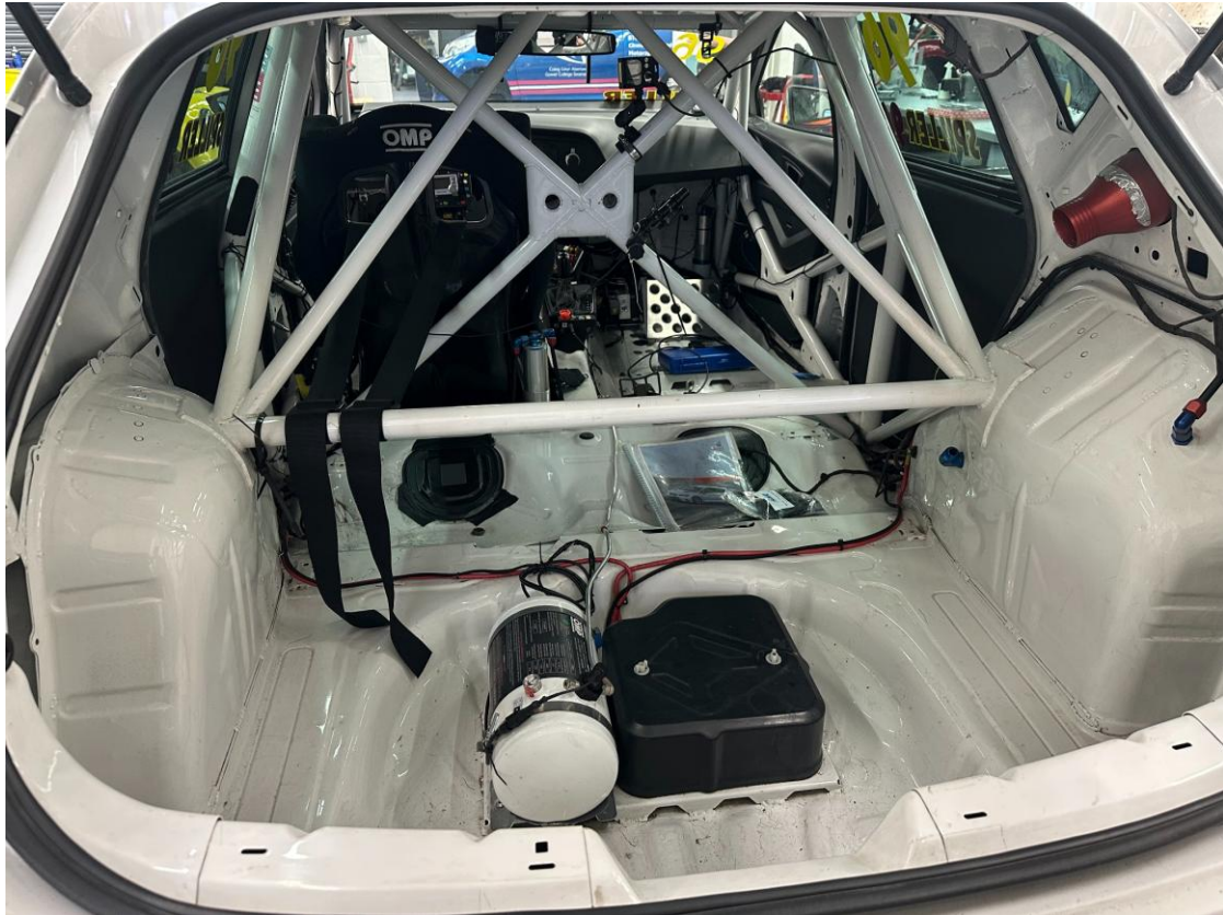
Figure 2. Cage triangulation and shell attachment at the rear of the vehicle, highlighting the additional load paths created to enhance rigidity.
