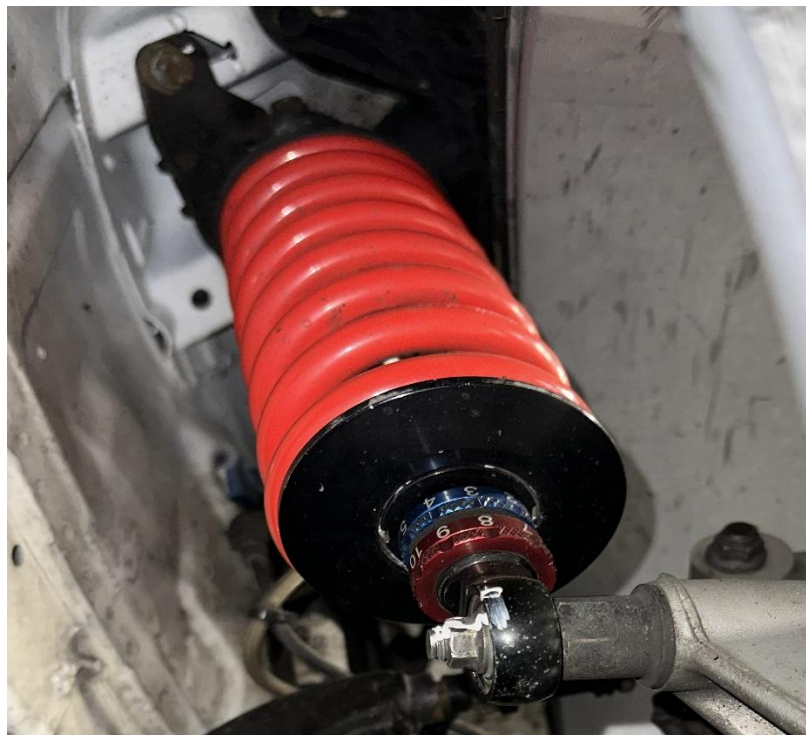
Figure 5. Rear suspension mounting area and wheelhouse, showing the rear load-path region where motorsport suspension forces are transferred into the production-derived shell.
