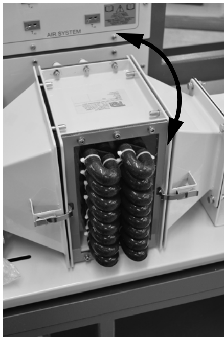
Figure 18 Heat Exchanger Fitted Backwards for Transport
