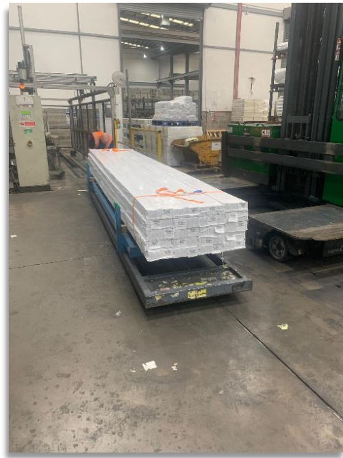
Fig.4 Operator pushing profile from outfeed
