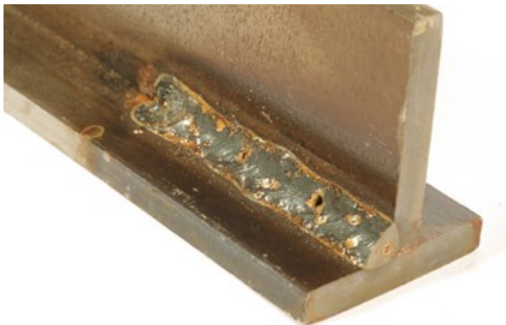
FIG. 1. No Shielding Gas on Steel - A lack of or inadequate shielding gas is easily identified by the porosity and (pinholes) in the face and interior of the weld.
