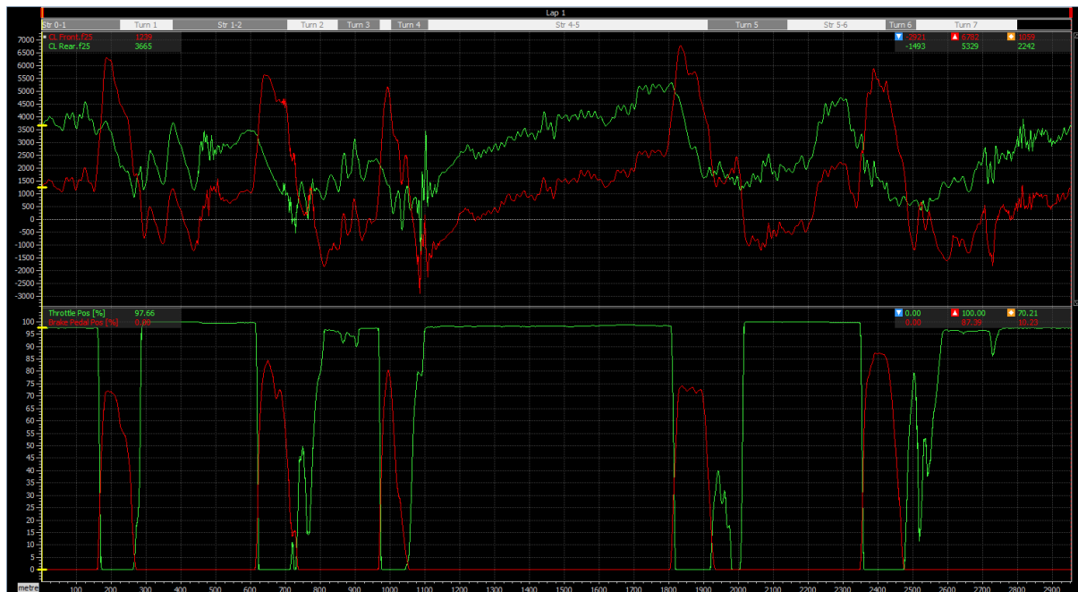
Figure 21 - Front and Rear downforce with throttle and brake position
