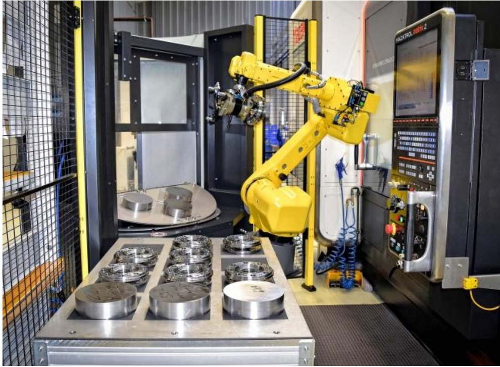
Figure 1. Automated loading and unloading of CNC machine tool (Zenoot, 2026).
