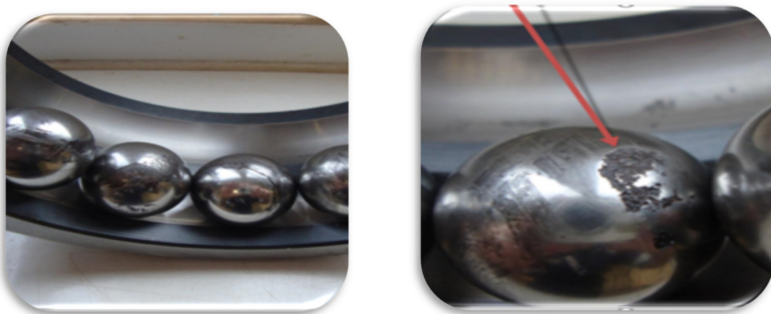
1.2.7 - Figure 10 – Ball Bearing Visible Defects (also highlighted in survey)
