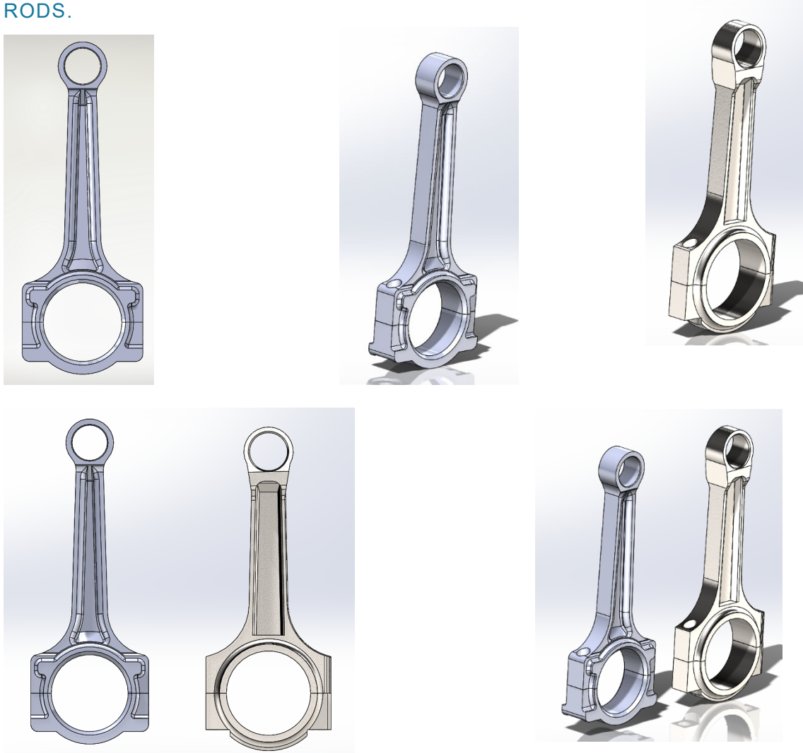
Figure 4 - Comparison of Ford connecting rods.
