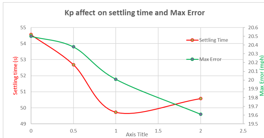
Figure 11 Kp effect on settling time and max error
