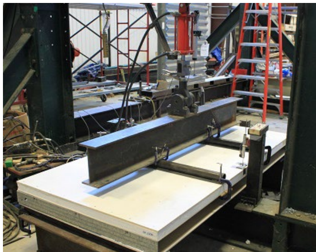
Figure 5: This image shows an example of beam deflection testing for a simply supported steel I-beam. The load is being applied by a hydraulic press with instrumentation attached to measure the deflection.
