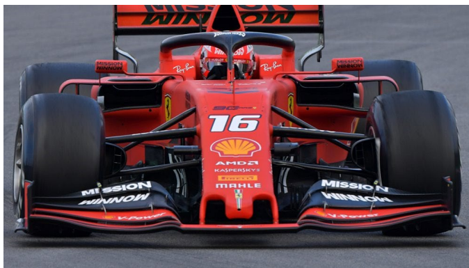
Figure 1: This image shows the front wing of the Ferrari SF90 2019 Formula 1 competition car. This is a common example of modern multiple element automotive front wing (Hughes, 2019).
