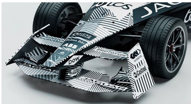
Figure 2: This image shows the front wing of the Jaguar 3 rd Generation Formula E competition car. This design has a unique double tier robust structural design (Attwood, 2022).
