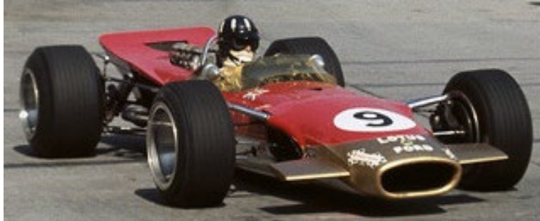
Figure 3: First automotive front wing introduced onto Graham Hills Lotus, Monaco 1968 (Oggioni, 2019).
