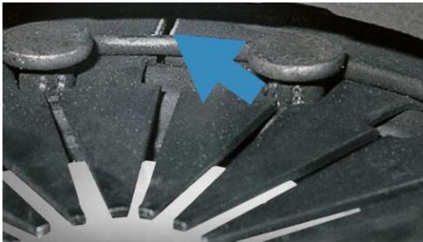
Figure 18--Fractured Diaphragm Spring from Fatigue (Performance GMBH, n.d.)
