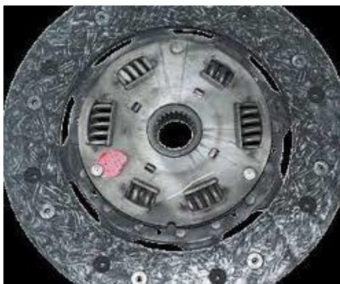
Figure 14-Example of Glazed Clutch Disk (Schaeffler, 2017)
