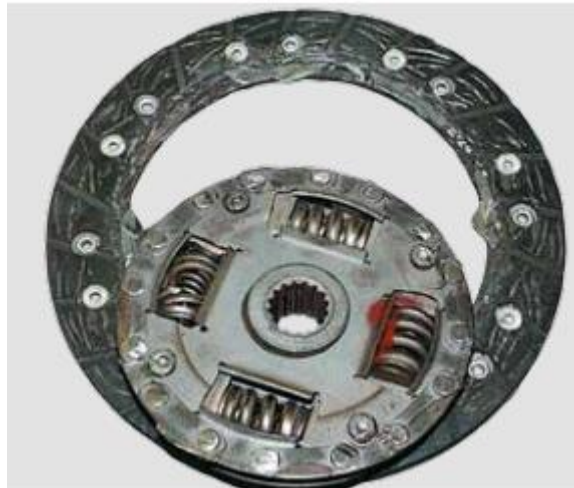
Figure 8-Example of a Fractured Clutch Disk (Schaeffler, 2017)
