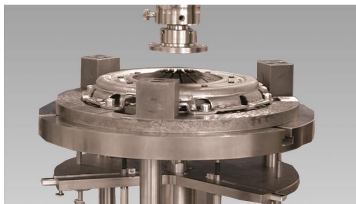
Figure 21-Fatigue Testing Machine for Diaphragm Spring (Zwick Roell, 2021)
