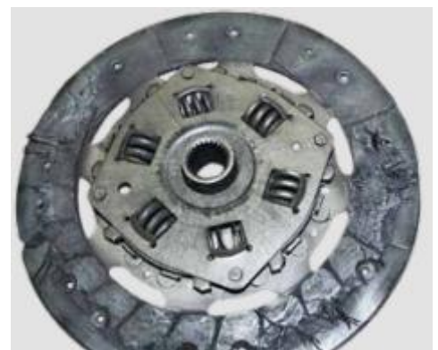
Figure 13-Example of Burnt Clutch Disk (Schaeffler, 2017)
