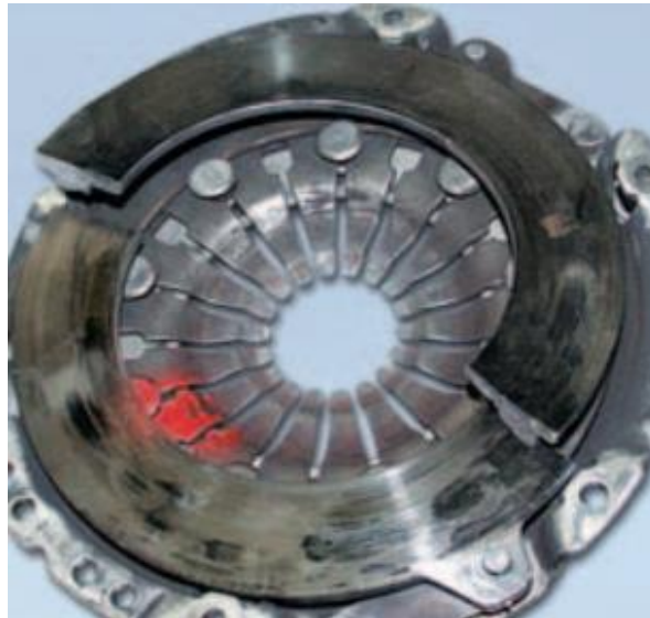
Figure 17-Example of Fractured Pressure Plate Due to Overheating (Schaeffler, 2017)
